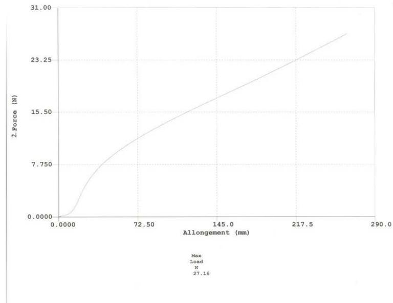
Via the notebook "AAElasticiteNonLineaire.nb" ( check the command: NotebookOpen[ToFileName[setdirectory,"AAElasticiteNonLineaire.nb"]] ) we have digitalized the above experimental non-linear curve to obtain a list of data ( evaluate the cell called "DIN").
