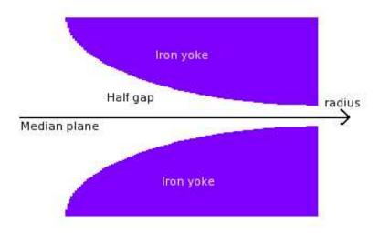
The second way to produce this field is to design a dipole with flat poles, and add series of conductors to the poles. Each conductor have its own current intensity.
