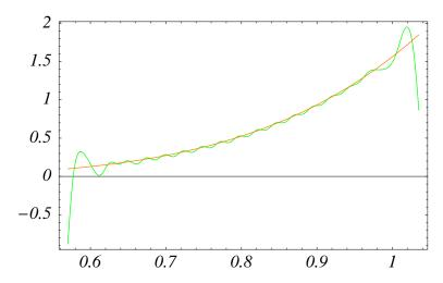
20 conductors in one plane or 40 conductors in two planes (green curve) and the theoretical field (orange curve).
