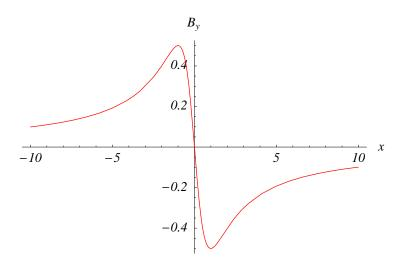
Let n be zero, if the gap is 1 then the maximum is located at x = -1 with amplitude 0.5 T, and the minimum at x = 1 with amplitude -0.5 T (see graph above).
