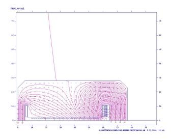
The picture above is the result of a *Poisson* calculation. The yoke is the zone where field lines are concentrated. The small squares are the conductors. The vertical field component profile along the ring radius is shown in the graph below.
