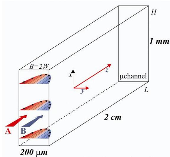
Figure 1. Microchannel scheme with dimensions used in simulations.
