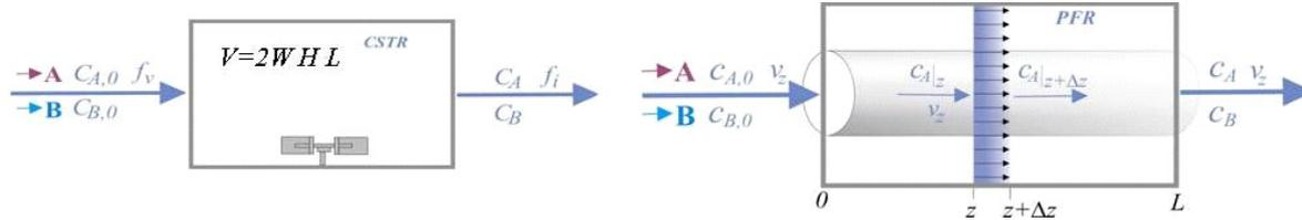
Figure 9. Schematic review of "microreactors" imitated the ideal behavior of *PFR* and *CSTR*.
