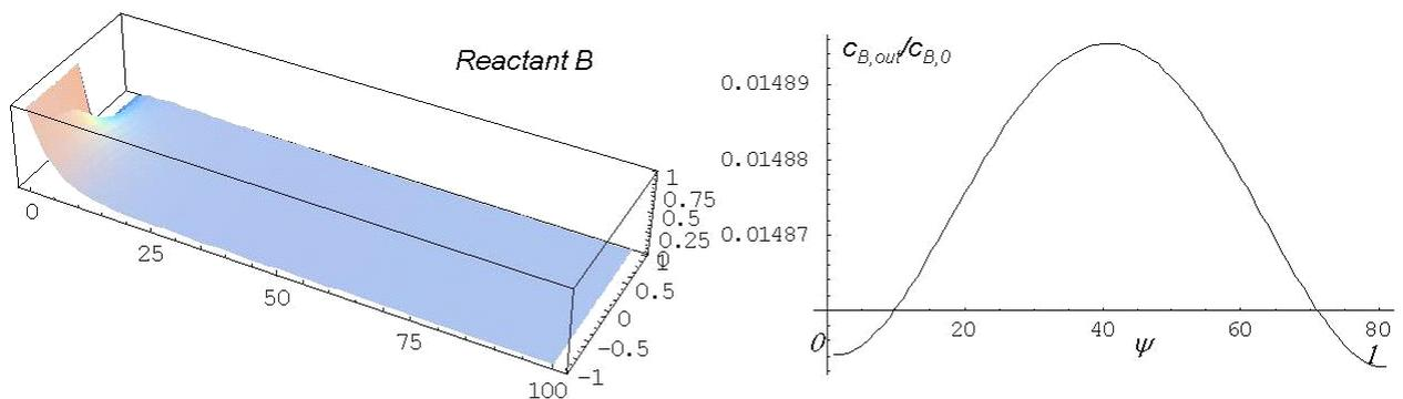
Figure 8. Steady-state dimensionless concentration profile in microchannel with the outlet profile of the reactant  $B$  ( $v_{av} = 0.001$  m/s;  $D_A = 1.1 \cdot 10^{-9}$  m<sup>2</sup>/s;  $D_B = 1.1 \cdot 10^{-8}$  m<sup>2</sup>/s;  $k = 0.9$  m<sup>3</sup>/kmol s).
