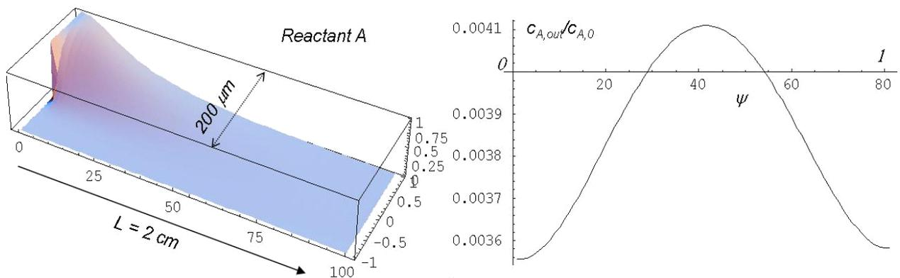
Figure 7. Steady-state dimensionless concentration profile in microchannel with the outlet profile of the reactant  $A$  ( $v_{av} = 0.001$  m/s;  $D_A = 1.1 \cdot 10^{-9}$  m<sup>2</sup>/s;  $D_B = 1.1 \cdot 10^{-8}$  m<sup>2</sup>/s;  $k = 0.9$  m<sup>3</sup>/kmol s).
