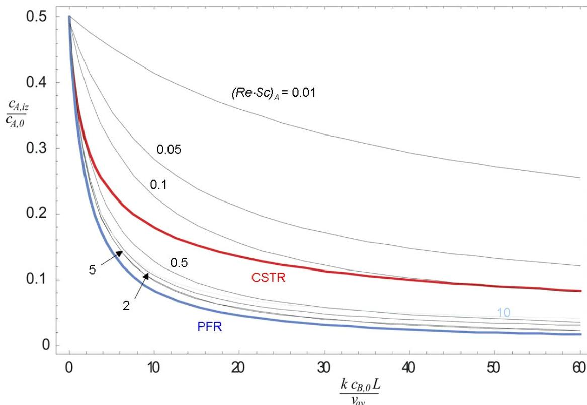
Figure 10. Comparison of the predictions of ideal *PFR* and *CSTR* models together with microchannel model simulations for a wide range of theoretical operating conditions, expressed as different  $Re \cdot Sc$  numbers ( $0.01 < Re \cdot Sc < 10$ ).
