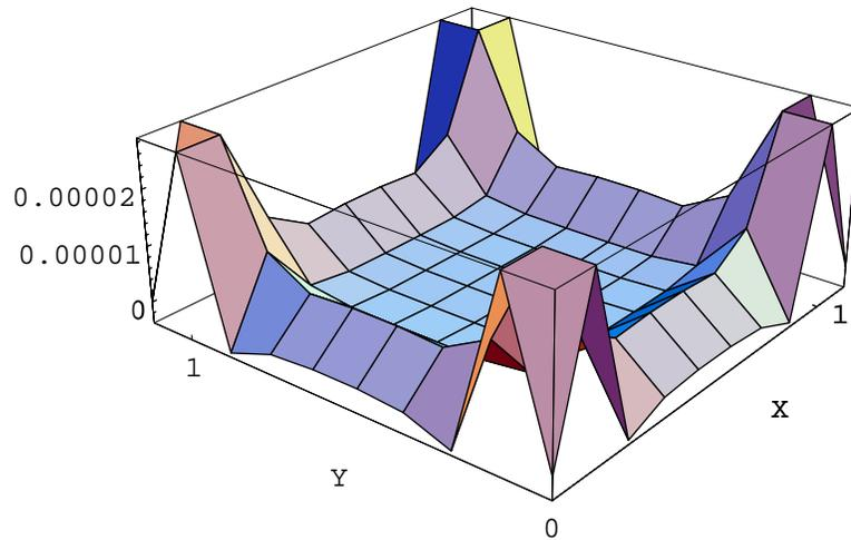
Figure 4 shows relative error of right-hand side function interpolated by RBF. Error of order  $10^{-5}$  points a very good approximation of right-hand side function.
