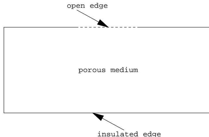
The reservoir is rectangle with edge of length  $2a$  and  $b$ . The open edge has length equal to  $2c$ . Because of symmetry of geometry and phenomena, the half of region will be considered. Figure 2 presents the geometry of the region taken into account.
